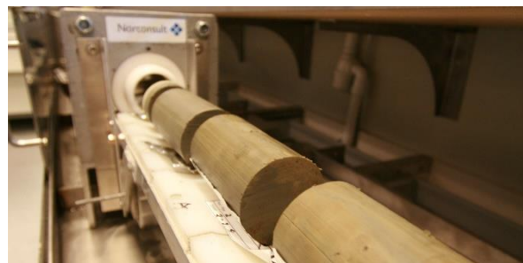
Figure 6 an undisturbed 54mm soil sample after ejection and cutting. Each piece is approximately 10cm long.
